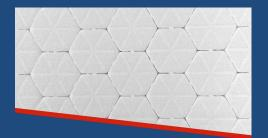
The 3D|CORE™ PET FR is a closed-cell, thermoplastic and recyclable rigid foam with excellent fire retardant, self-extinguishable properties according to EN 45545-2 and IMO 2010 FTP Code Part 5. The honeycomb structure provides more flexibility and is easy to handle easy to handle.
